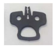
A quick note on assembly: your Omega has hydraulic brakes, and includes a spacer in the front brake caliper to keep the brake pistons retracted. This must be removed prior to assembly, and should be installed when the front wheel is removed. The caliper is located at the bottom of the front fork. Simply pull the plastic tab out to remove it, and slide it back in after wheel removal:
