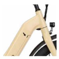
**Note:** The battery can be charged on or off the bike. To remove the battery, insert and turn the key on the left side of the battery, then lower the battery away from the key at the top. To install, insert the battery at the bottom and swing back into position while pushing up towards the frame. Turn the key to lock the battery in place
