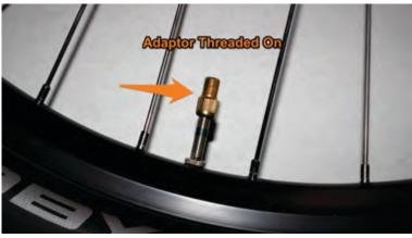
To release air, depress the valve core.
