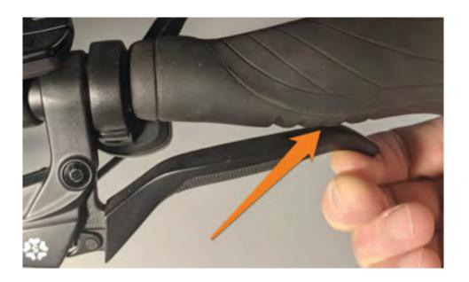
The solution is to increase cable tension in the system. This can be done without tools and possibly even when you are out on a ride.
