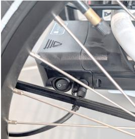
We recommend against passing the charging cable through the wheel, even though it may be easier. If you forget to unplug the charger and move the bike, it will likely damage the charger.
