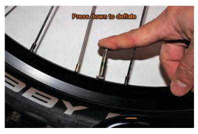
Be sure to tighten the captive nut after making your air pressure adjustments.
