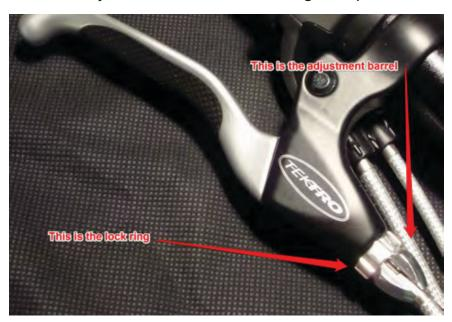
First, loosen the lock ring by unscrewing it so there is a slight gap between it and the lever mount.
