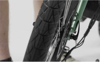
Remove the fender mounting bolt/washer from the right side of the fork.
