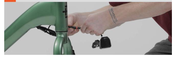
Attach headlight and fender assembly to fork. Position the fender as high up as possible and tighten the bolt and nut.
