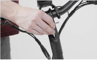
Align handlebars to front wheel then snug up the headset preload bolt, so that the spacers below the stem do not rotate easily.
