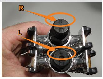
It is important to note that the pedals are threaded differently. The right pedal will be on the same side as the chain and screws in clockwise. The left pedal goes on the side without the chain and screws in counterclockwise.
