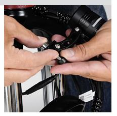
Attach Headlight and Fender assembly to fork.
