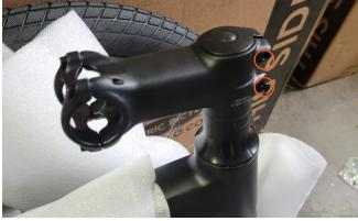
Remove the 4 screws on top of the stem faceplate.
