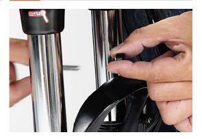
Thread Headlight and Spacer onto screw.
