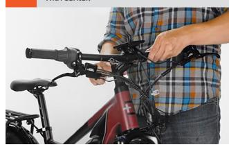
Replace cover and the 4 screws on top of handlebars.
