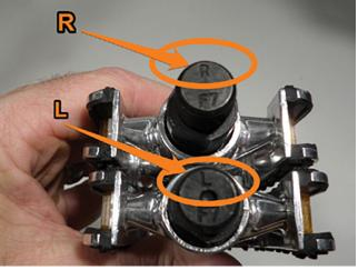
It is important to note that the pedals are threaded differently. The right pedal screws in clockwise and the left pedal screws in counter-clockwise.
